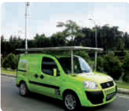
StarHub introduced Singapore's first solar-powered cellular BTS-enabled vehicle, the Mobile 'Greenery' vehicle.
